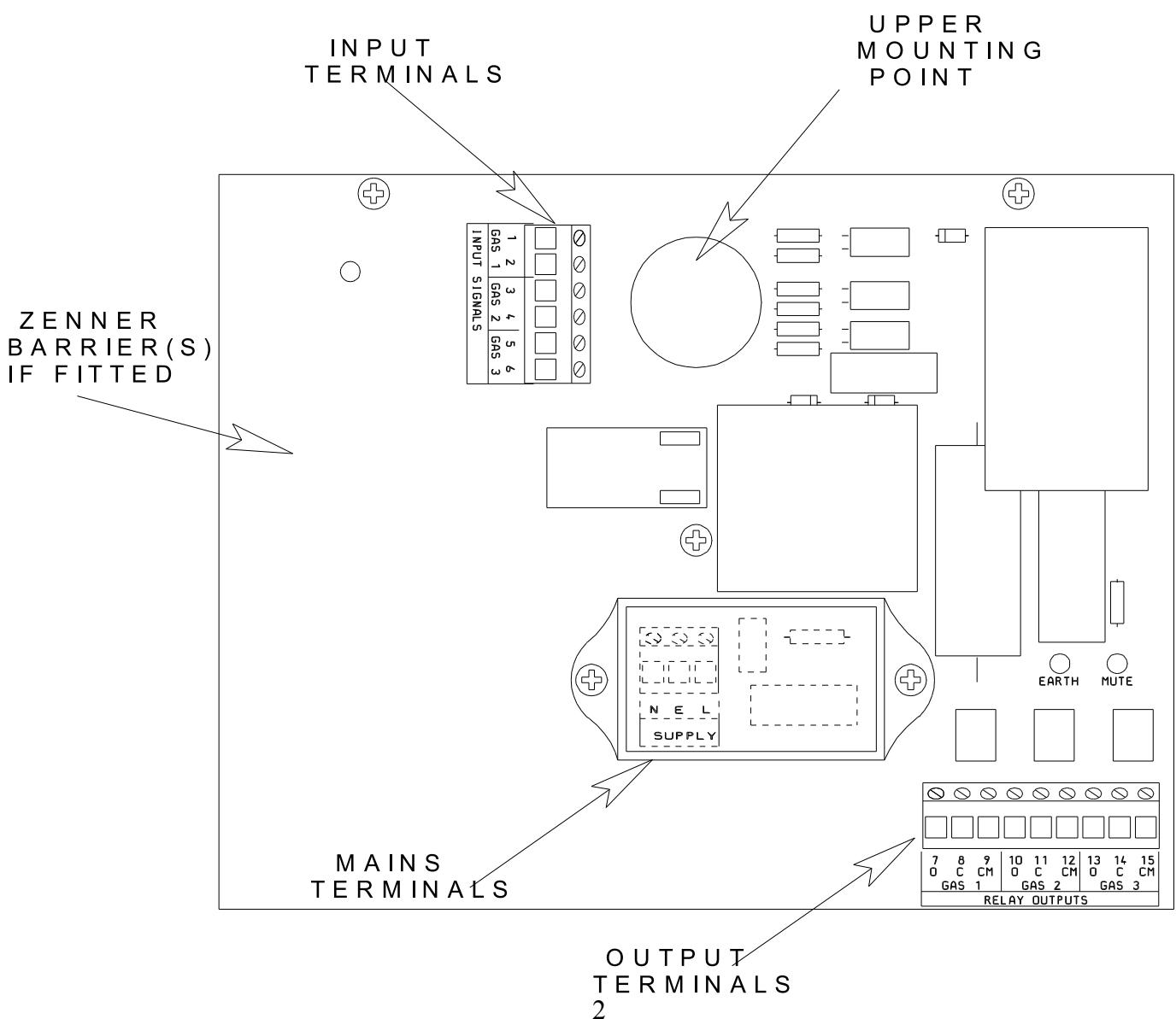
Cable entries should be made on the lower edge of the Terminal Chamber. Remove the Mains Terminals cover. Connect a 240 v ac supply, fused at 3 amps, to the L, E & N terminals. Make a cutout in the side of the Mains Terminals cover to clear the cables and replace the cover. Connect the input devices and output relays (if used) as shown on the drawing accompanying the alarm panel.
