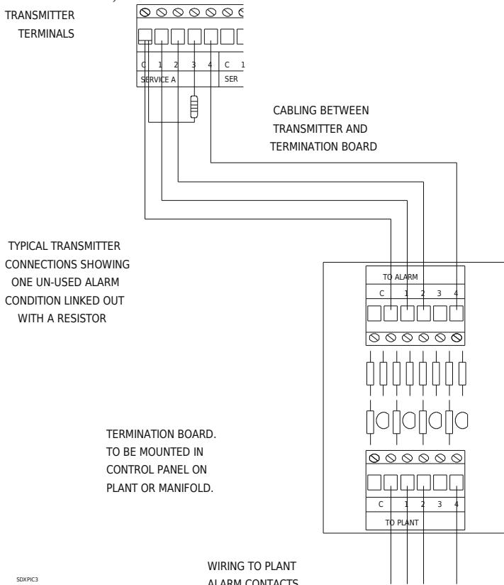
Any condition not transmitted from this transmitter must be terminated with a 56k resistor to set the condition to normal if the condition is not to be used, or with a 1k8 resistor if the condition is to be transmitted from another transmitter. The resistors are used to prevent a system fault due to short or open circuit. Note that if a resistor is fitted, the condition must NOT be connected to the termination board.
