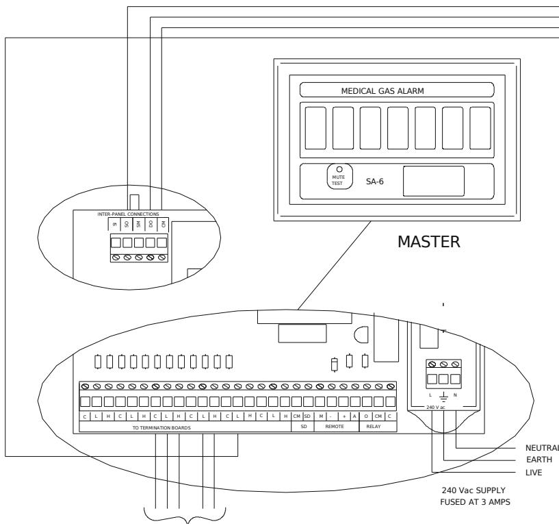
Connections to pressure switches when termination boards are used.
